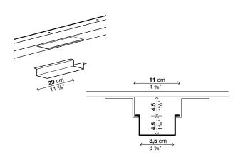
Under-top tray in transparent methacrylate. It slots into the openings of the central drawn element of the structure and houses electric gang-sockets.
