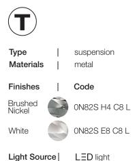
Input: 100-277 Vac. 50/60Hz Dimmable 1 - 10V Total output - 3590 lumen Color temperature - 3000 K Color accuracy - 80 CRI Total nominal power consumption - 31,5 Watt Power supply included in canopy TERZANI LA LUCE PENSATA
